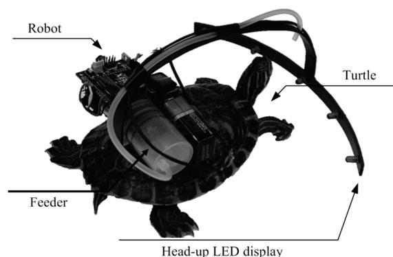
**Fig. 2** The parasitic robot is mounted on the carapace of the turtle. It induces the turtle to move to the waypoint by using a head-up Light Emitting Diode (LED) display as well as rewarding the turtle with food when it performs well.
