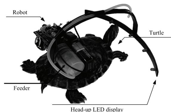
**Fig. 2** The parasitic robot is mounted on the carapace of the turtle. It induces the turtle to move to the waypoint by using a head-up Light Emitting Diode (LED) display as well as rewarding the turtle with food when it performs well.
