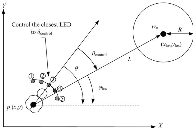
**Fig. 4** Guidance algorithm for the parasitic robot from the  $(n-1)$ th to  $n$ th waypoints. The parasitic robot gets data on the position of the turtle and waypoint, and controls the lit LED (virtual target point) with a line of sight guidance algorithm.
